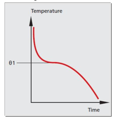
$\theta$ 1 is the temperature at which the solidification begins  $\theta$ 2 is the maximum temperature reached at the end of the undercooling  $\Delta\theta$  is the apparent undercooling equal to  $\theta$ 2- $\theta$ 1 t1 is the duration of undercooling.
